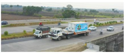
Liquid nitrogen based Reefer undergoing road trials
