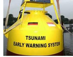
The Indian Tsunami Early Warning Centre (ITEWC) set up by MoES at the Indian National Centre for Ocean Information Services (INCOIS), Hyderabad (left) and a buoy moored in the ocean for collecting data on tsunamigenic earthquakes (right)
