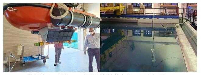
Fig. 3.17 (a) Assembled Prototype i-SASSS A (b) Digital hydrophone array during ATF tests
