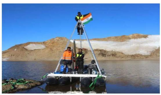
Fig. 4.2 Retrieval of two sediment cores from Discussion Lake, Broknes Peninsula (East Antarctica) using a VibeCoreD4 corer on a UWITEC platform during the 41<sup>st</sup> Indian Scientific Expedition to Antarctica.
