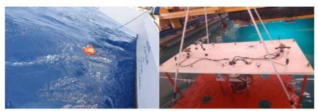
Hg. 3.18 (a) Deep Water Ambient Noise System Deployment in Arabian Sea (b) Field trial of Bottom mounted vector sensor system
