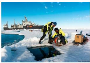
Fig. 4.8 Photo showing an NCPOR team member deploying a turbulence profiler for studying the ocean turbulence in the Central Arctic Ocean and R.V KronPrinsHakoon is seen in the background.
