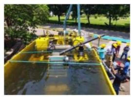
7.1 Self-propelled Miner and integrity tests in a Water Test Tank
