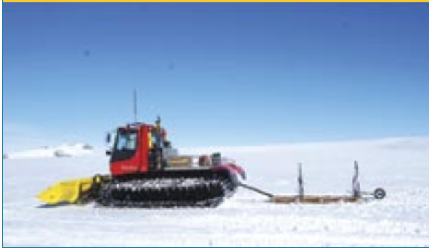
Fig. 4.3: GPR profiling on Polar Ice Cap with 35MHz antenna
