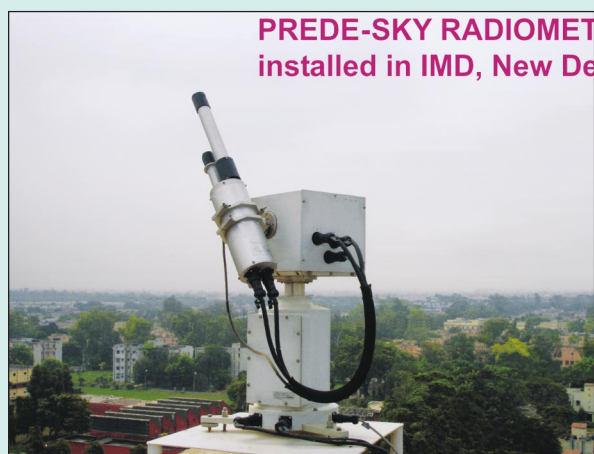
Sky radiometer installed to monitor the impact of atmospheric aerosol on Radiation balance.
