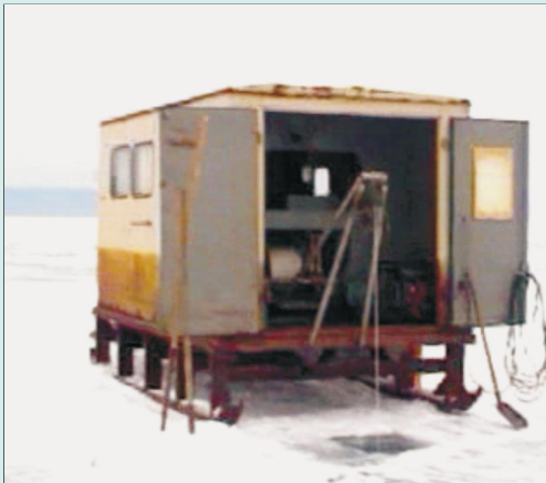
Deployment of Methane sensor
