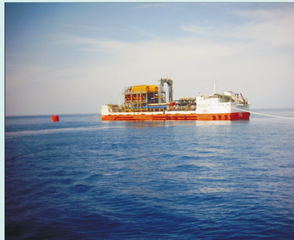
View of the barge "Sagar Sakthi" connected to the Single point mooring buoy at 1000 m water depth off Ennore port.
